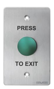
Panel: Stainless steel, 304 grade, 1.7mm thick, laser etched text Dimensions: 115H x 70W x 37D (mm) Button Colour: Green Output Contact: 1x NO & 1x NC Mechanical Life: 500,000 Operations Ingress Rating: IP65 Contact Rating: 12-24V DC / 0.5A Operating Temperature: -20°C to +70°C **Operating Humidity:** 0-95% (relative humidity) **Weight:** 145 g Fixing Method: 2x3mm stainless steel screws (included) Mount Style: Flush - fits Australian wall boxes
